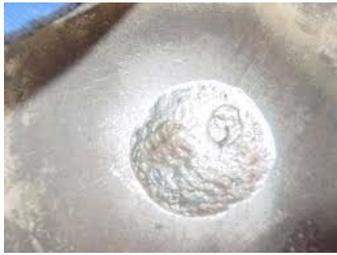
AC corrosion occurs where overhead power lines are located parallel to a buried pipeline. AC potentials can be electromagnetically induced into the pipeline and corrosion occurs where the potentials leave the pipeline to return to the source.
