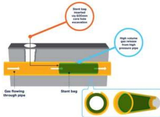
The Stent Bag (Stage 2) is currently in development focusing on gas escapes on pipe systems with Maximum Operating Pressure (MOP) up to 7 barg and up to 12" PE and metallic pipelines. This offers a safer alternative than conventional means and also maintains security of supply to our customers downstream of the incident. The stent equipment can also be used to remediate bolts found on AVK valves, providing further safety compared to conventional methods.
