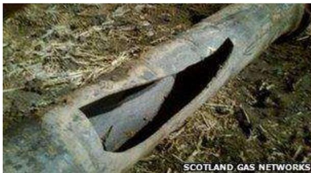
Depending on the extent of the damage, the first choice option for dealing with third party damage is to try to maintain the gas supply to customers. The current method for achieving this is to temporarily repair/ control the leaking pipe with a repair clamp and/ or sandbags and then construct a bypass around the damage, subsequently cutting out the damaged section. An example of current techniques can be seen in Error! Reference source not found..
